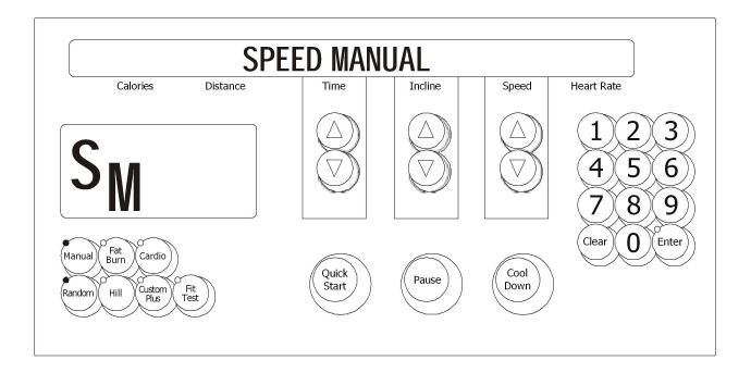
Upon entry into this test the letters SM (Speed Manual) will be in the profile window. This test allows the user to test the main drive motor and controller controlling the motor rpm. The user can select a target motor rpm by using the speed arrow keys. The actual motor rpm as calculated by the speed feedback sensor is shown in the actual portion of the message center.
